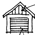
SIMPLE GABLE TREATMENT DOORS TO BE SIMPLE TIMBER OR METAL CLADDING - NOT PANELLED 'PANCY' DOORS
